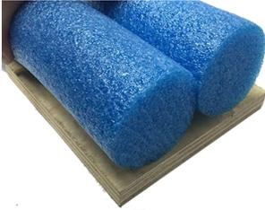
**Step 9:** Wrap fabric tightly around noodles. No noodles should be showing after wrapping. Staple fabric evenly along edge of bumper and trim any extra fabric. You will need to access the holes and hardware to attach bumpers frequently.
